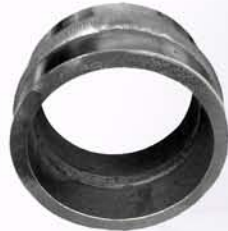
Example of Pipe Weld: 4" Carbon Steel, Sch 80
