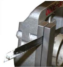
Pictured: example using Saw Guide to cut pipe/tube
